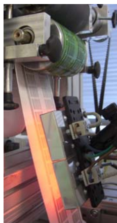
Source and drain printed with flexography. The silver ink is sintered online using IR radiation
